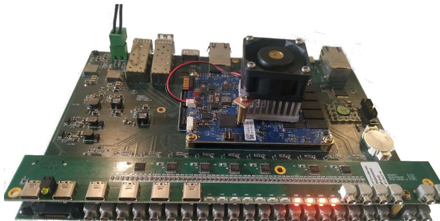
Figura 2 – Photo of Gaugit DC16B1250 multichannel digitizer boards with ZU7EV SOM board from iWave Systems.
